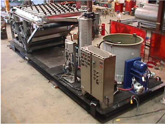
In some applications it may be necessary to separate larger grained materials from finer grained materials. Eagle utilizes a combination of hydro cyclones, high frequency screens, and settling tanks.
