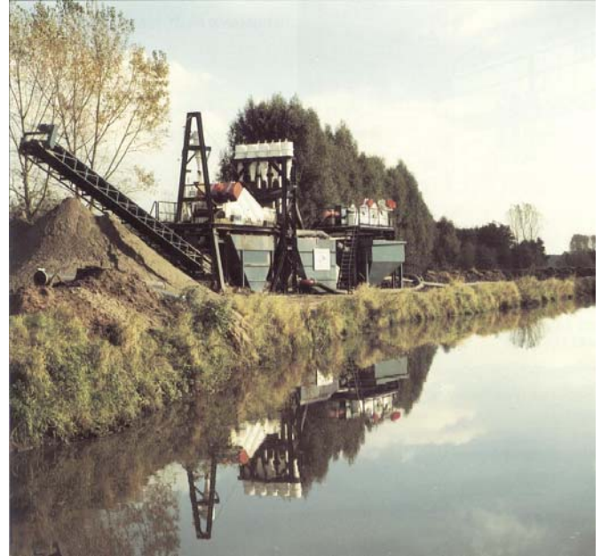
In some applications it may be necessary to separate larger grained materials from finer grained materials. Eagle utilizes a combination of hydro cyclones, high frequency screens, and settling tanks.
