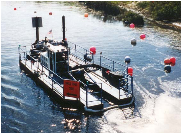
Adak is an 8" cutter suction dredge specially designed to operate in narrow canals and rivers.
