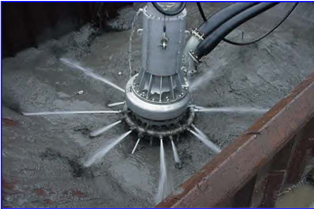
Eagle's 75 Hp TOYO Pump operating with high-pressure jet-ring. The TOYO Pump is the most aggressive solids pumping pump set available in the world. It is capable of pumping 5 ½" rocks and debris, with a solids content in excess of 35% solids
