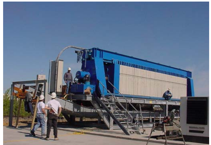
Eagle's 12.5 Cubic Yard Membrane Squeeze Plate and Frame Filter Press being set up for operation at a remote location in Canada.
